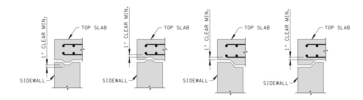
NOTE: WHEN ALTERNATE JOINT DETAIL IS PROVIDED, MINIMUM CLEAR DIMENSIONS AND INTERIOR SLAB THICKNESS SHOWN ON STANDARDS SHALL BE MAINTAINED.
