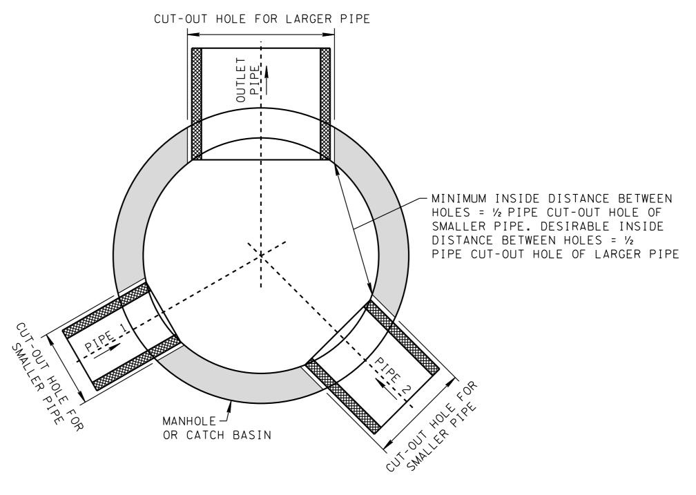
NOTE: IF SMALLER PIPE IS AN UNDERDRAIN, A 6" MINIMUM INSIDE OFFSET FROM AN ADJACENT HOLE IS REQUIRED. OFFSET MAY BE HORIZONTAL OR VERTICAL. UNDERDRAIN CONNECTIONS SHALL BE LOCATED A MINIMUM OF 8" BELOW THE BOTTOM OF THE TOP SLAB.
